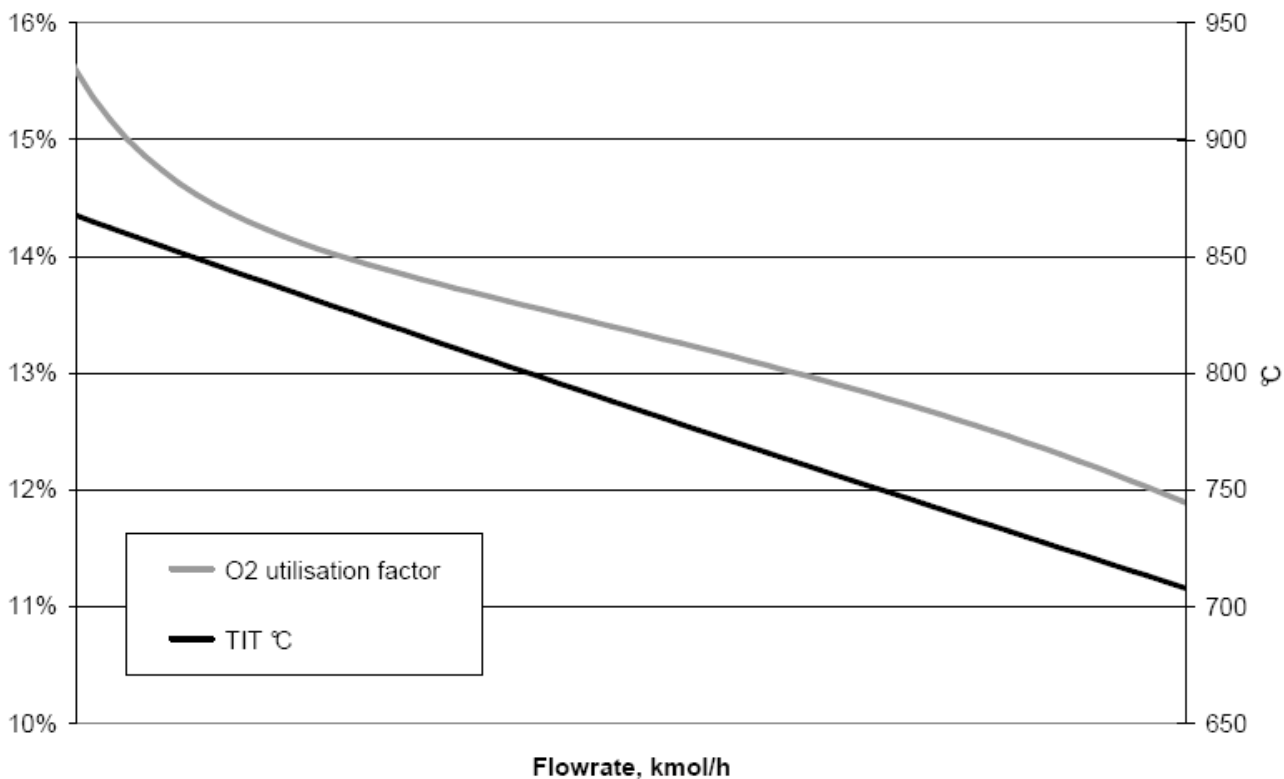
Figure 4 – Effect of the feed flow-rate of fuel to the FCS on the oxygen utilisation factor and the turbine inlet temperature at the nominal operating pressure.
